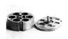
Specimen Container with 6 chambers 0 10 x 14 mm and 3 chambers 4 x 6 x 14 mm to accept up to 9 different specimens. All specimen chambers can be closed with a common cover of fine wire mesh. For suspensions, filter paper can be used instead of the wire mesh.
